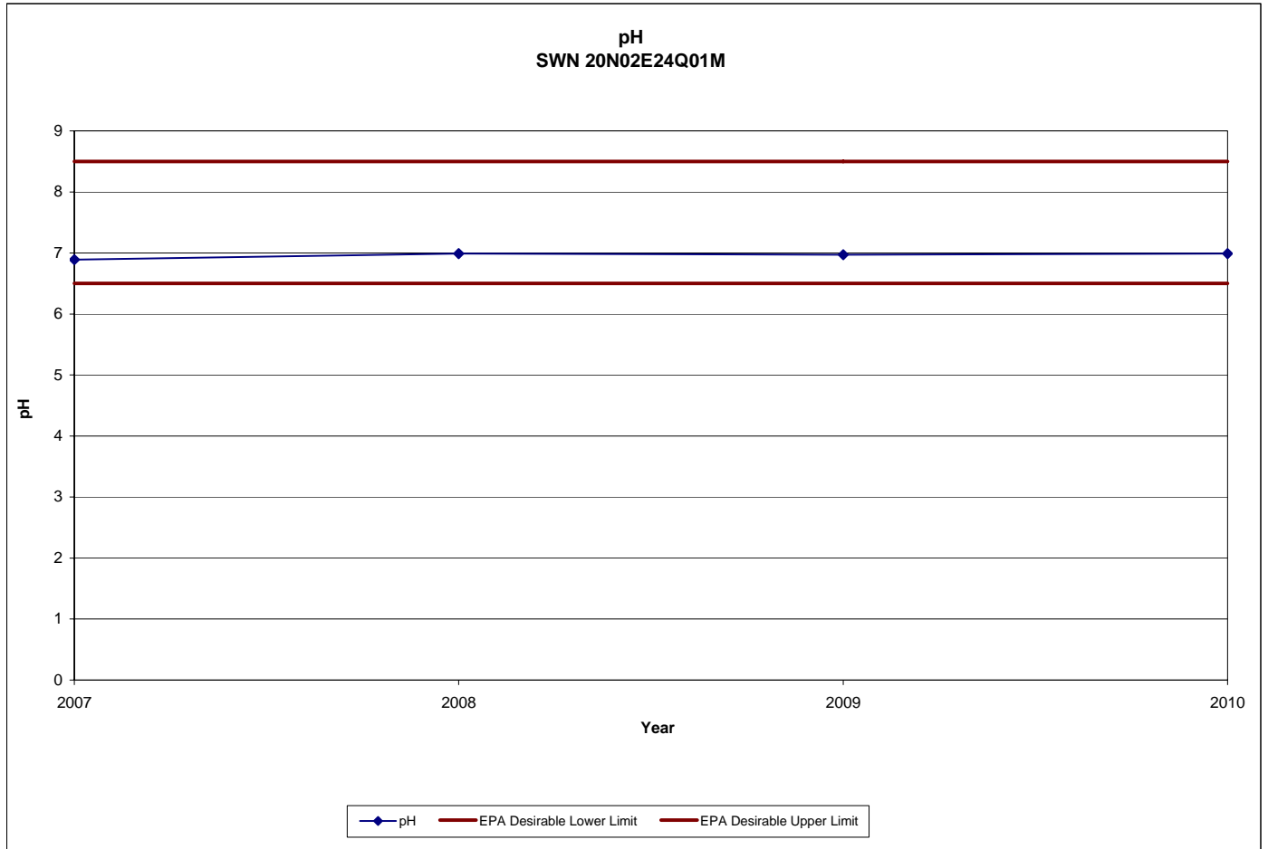
Figure 7. Chico Urban Area well monitored for pH
