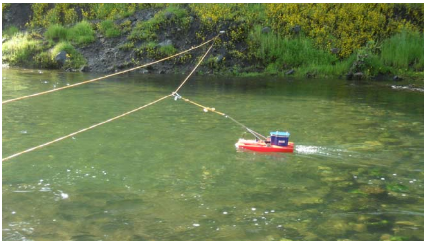
Figure 7. Field Test of StreamPro ADCP at Big Chico Creek
