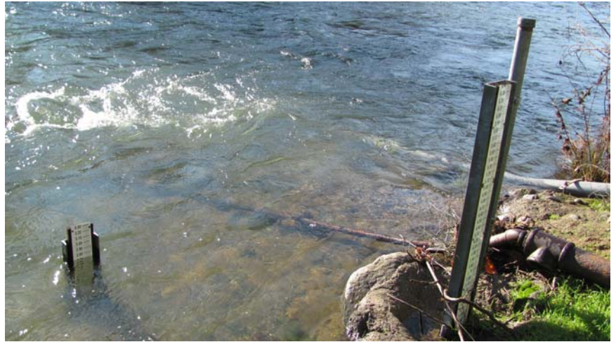
Figure 5. Existing Staff Gauges within Butte Creek
