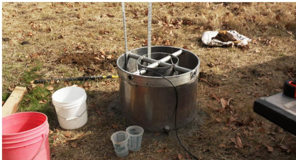
Figure 6. Dual Ring Infiltrimeter Testing – SD-IR-12
