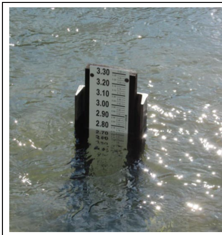
Figure 3: Stream Gauge (Photo)
