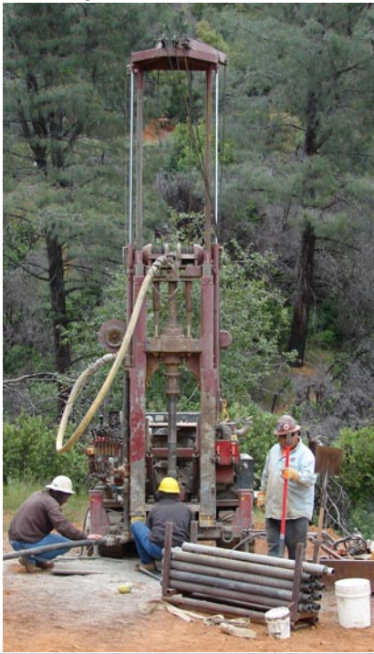
Figure 4: Limited Access Mobile Drill Rig (Photo)
