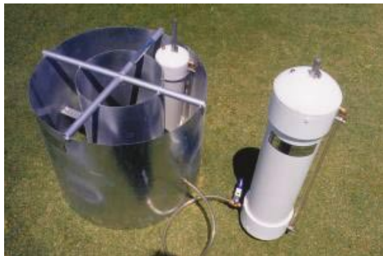
Figure 2: Dual Ring Infiltrometer (Photo)
