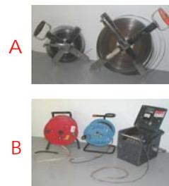
*Typical devices to measure groundwater levels:*
